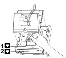
Attach the line cord to jack number 2 and the other end to the modem or fax machine. This line cord is not supplied with the telephone.
