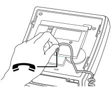
Attach one end of the handset cord to the handset and the other end to the handset jack.
