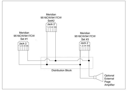
**Note**: A separate jack and a 6 conductor line cord is required to connect page lines. This cord is not supplied with the 9516CW telephone. Contact your telephone company representative to have page lines connected to your telephones.
