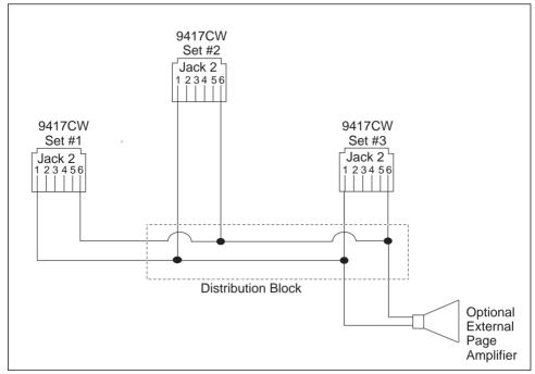
**Note**: A 6 conductor line cord is required to connect page lines. This cable is not supplied with the 9417CW telephone. Contact your telephone company to have page lines connected to your telephones.
