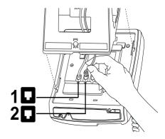
Insert the first line cord in jack 1 as shown by 1 . Insert the second line cord in jack 2 as shown by 2 . Insert the other ends of the line cords into the wall jacks.
