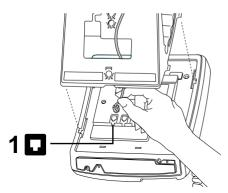
Insert the line cord in jack 1, as shown by 1 . Insert the other end of the line cord into the wall jack.
