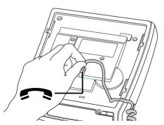
Attach one end of the handset cord to the handset and the other end to the handset jack.
