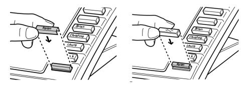
After programming the memory keys, label them with the supplied blank labels and key caps.  $^{\dagger}$
