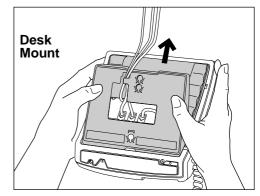
Lower the stand into the slots on the base of the telephone, as shown in the desk mount illustration above. Slide the stand back until it clicks into the locked position. The excess line cord fits into the stand of the telephone.
