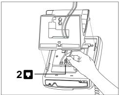
For your fax machine, answering machine or modem; attach the line cord in jack number 2 as shown by 2 .
