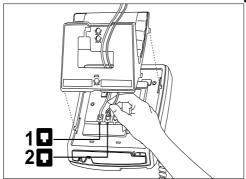
Attach one end of the line cord to jack number 1 and the other end to the wall jack. Attach the second line cord to jack number 2 and the other end to the wall jack. Both line cords are supplied with the telephone.
