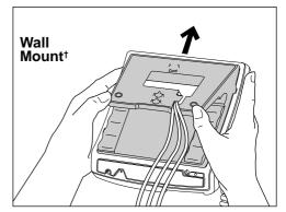
Lower the stand into the slots on the base of the telephone, as shown in the wall mount illustration above. Slide the stand back until it clicks into the locked position. The excess line cord fits into the stand of the telephone.
